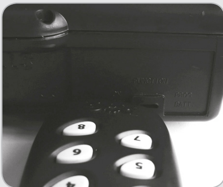
Position when turning the ball feeder on/off and when matching the transmitter with the ball machine.
